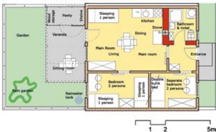
Drawing 3: Floor plan of a house with an apartment, a porch and a front lawn, designed according to the Ivanjica system
