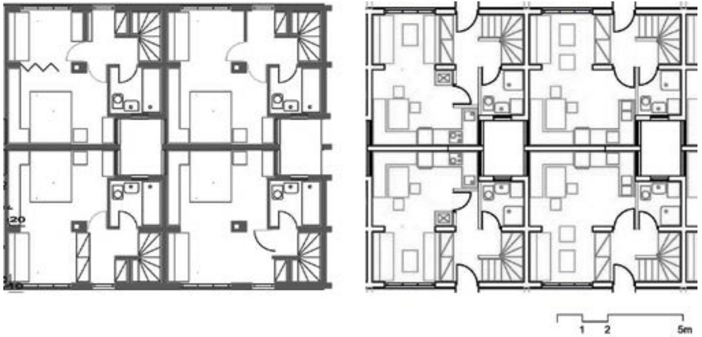
Drawing 43: SOLECO type incremental enlargement house evolving around the kitchen and a bathroom
